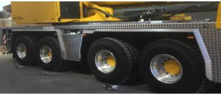
The *split rims* are different from regular single piece wheels found on cars and heavy vehicles because unlike regular rims, they are held together by bolts and/or a lock ring. This means that there is an extra interface where something can go wrong. Incidents involving split rims are still very common with 2 recent cases reported by Worksafe Victoria.
